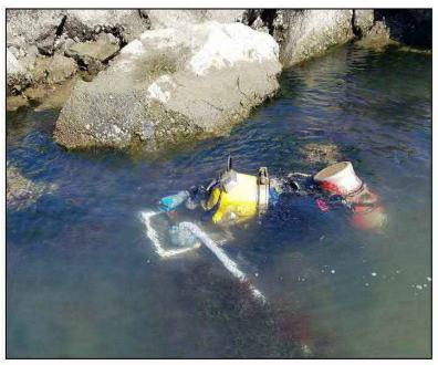
Figure E-3. Diver scraping the rock and suctioning the sample into a collection bag at a subtidal site during the portal island benthic survey
