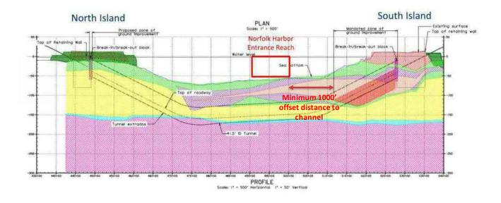
Proposed alignment for the bored tunnel between existing North and South Islands
