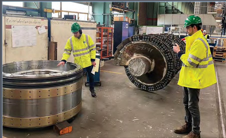
PHOTOS: (Left) A single bearing being constructed for the TBM in Germany.
