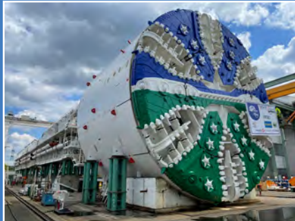
[ABOVE]: The TBM was fully assembled for the Factory Acceptance Test in Germany.
