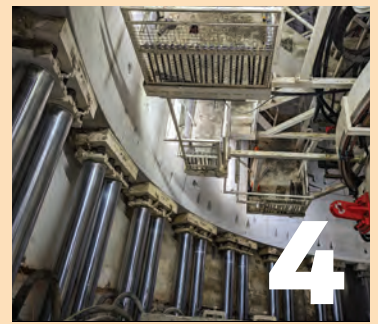
[ABOVE]: 1 The TBM operator monitors all operations from the control room. 2 Multi-service vehicles are used to transport the tunnel segments to the TBM. 3 The segment feeder brings in tunnel segments as the vacuum erector awaits overhead, preparing to move each segment into place. 4 The TBM has 54 hydraulic thrust cylinders that push against the tunnel ring to move the TBM forward.
