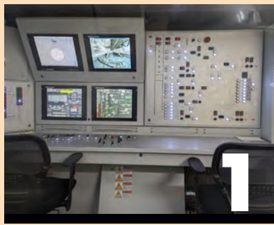
[ABOVE]: 1 The TBM operator monitors all operations from the control room. 2 Multi-service vehicles are used to transport the tunnel segments to the TBM. 3 The segment feeder brings in tunnel segments as the vacuum erector awaits overhead, preparing to move each segment into place. 4 The TBM has 54 hydraulic thrust cylinders that push against the tunnel ring to move the TBM forward.
