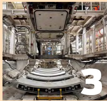
[ABOVE]: 1 The TBM operator monitors all operations from the control room. 2 Multi-service vehicles are used to transport the tunnel segments to the TBM. 3 The segment feeder brings in tunnel segments as the vacuum erector awaits overhead, preparing to move each segment into place. 4 The TBM has 54 hydraulic thrust cylinders that push against the tunnel ring to move the TBM forward.
